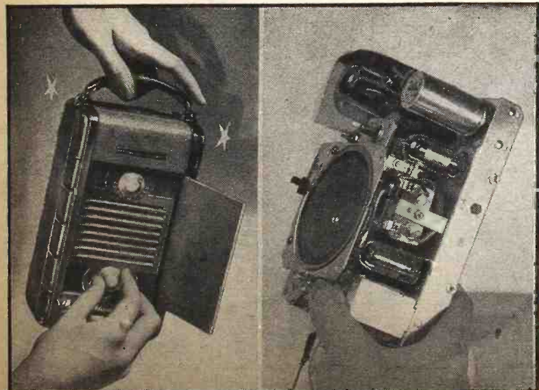
Front and rear views of the Admiral 28-G5 5-tube Battery/Electric Portable. Ventilation for the rectifier tube is provided at the top of the molded plastic case.
